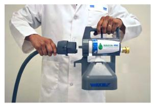
3.) Now make sure to properly align foam/ spray nozzle to locking tabs on dispenser before connecting
